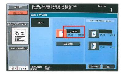
When keying in your selection, keep in mind the decimal place. For instance, if you would like a 75% reduction you will need to key in "750" on the keypad. If you only key in "75" then you are actually only setting the zoom to 7.5 which is outside of the allowable range of 25.0 - 400.0. Press the "C" button near the numeric keypad to clear the entry if needed. Press "OK" to return to the previous menu.
