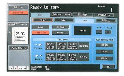
This zoom menu allows you to select preset reduction and enlargement settings. Use the "+" and "-" buttons to manually fine tune your zoom selection. (Note that this is only for very fine adjustments) To manually key in a reduction or enlargement ratio, press the "XY Zoom" button and key in your selection using the numerical keypad. By pressing the "XY Zoom" button, you will see a screen similar to that shown below.
