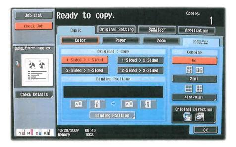
The "Binding Position" button will change the way the two sides are oriented to one another. Be sure to press "OK" to return to the previous menu.
